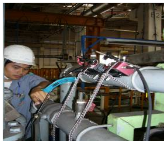
A-6 Flow rate of hot water outlet couldn't detection because of water was flowed by spot flow
