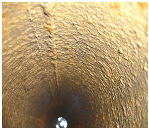
C-6 Scaling texture are still remaining same as the 60 days ago.
